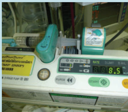
Image 3.1.7 Machine for dripping control of milk or intestinal nutrients
